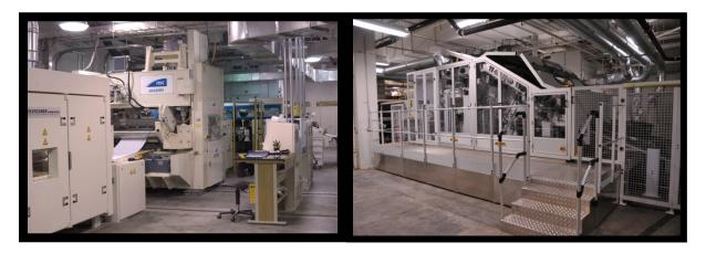
The Asselin "Profile 415-FD" crosslapper has automatic batt width adjustment, automatic overlap control and adjustment, and full control over the number of layers, with automatic computation of the necessary delivery speed on the floor apron. This equipment is capable of producing very light batts. The "Profile", as its name implies, is capable of shaping the outgoing material to optimize weight distribution from center to side of the fabric.
